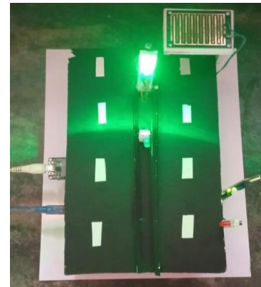
Fig. 2. Shows the implementation of Smart Street Light
