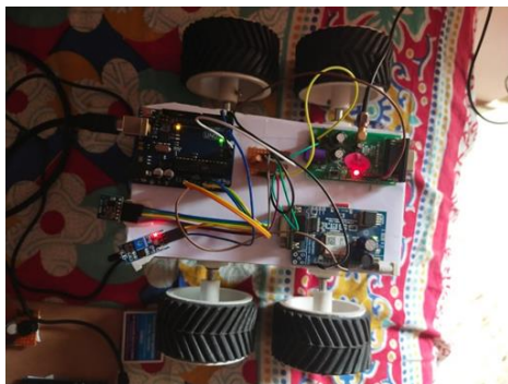
Fig. 4. Automatic Vehicle Accident Detection and Messaging System Using GSM and GPS Modem
