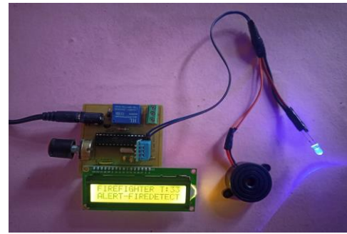
Fig. 3. Smart fire detection system
