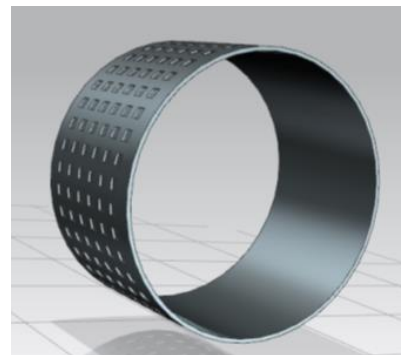
Fig. 15. 3-D Modeling of square geometry liner in Unigraphics N-x
