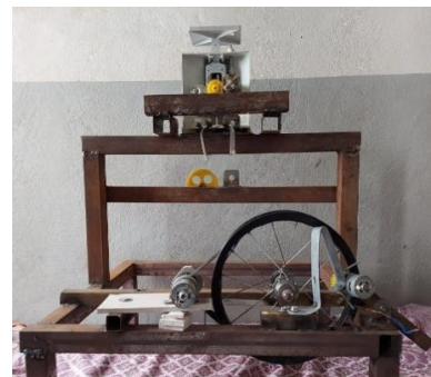
Fig. 8. Model of suspension and regenerative braking system
