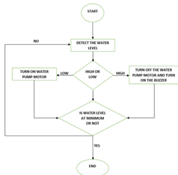
Fig. 1. Flowchart of water level detection system
