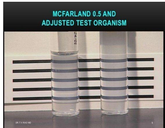
Fig. 5. 0.5 McFarland Standard turbidity ratio using Wickerman card background
