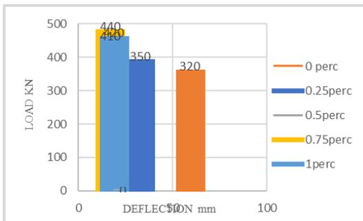
Fig. 20. L shape of BC joint BC joint comparing the results load v/s deformation without and with various percentage of PVAFRCCs
