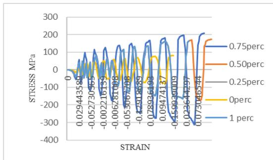
Fig. 19. LVDT shape of BC joint results stress v/s strain without and with various percentage of PVAFRCCs
