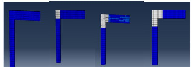
Fig. 10. PVA composite adding in L shape BC joint junction
