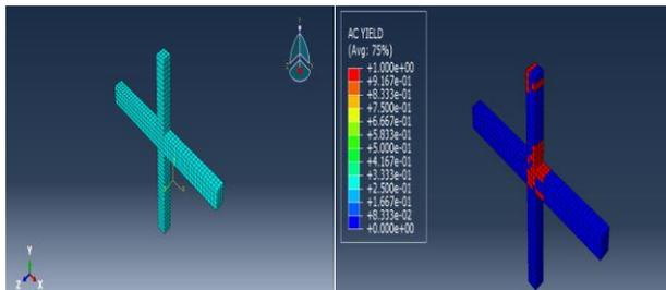
Fig. 6. Meshing and yielding of reinforcement and cracks in the model
