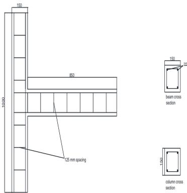
Fig. 1. T shape BC joint
