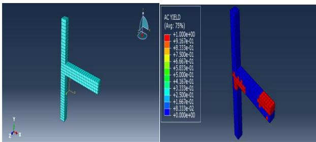
Fig. 5. Meshing and yielding of reinforcement and cracks in the model
