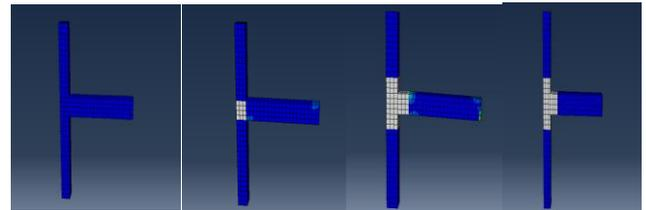
Fig. 8. PVA composite adding in T shape BC joint junction
