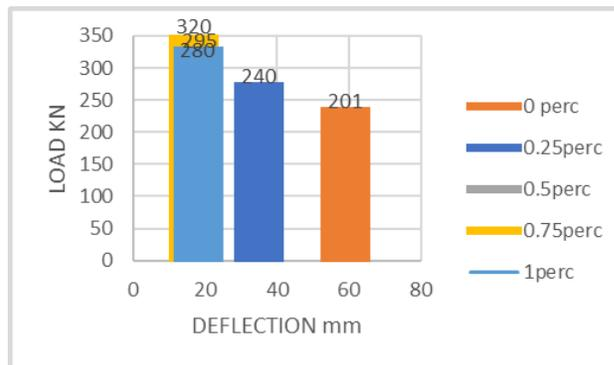
Fig. 18. Maximum load and minimum deflection of the without and with various percentage of IN PVAFRCCs LVDT BC joint
