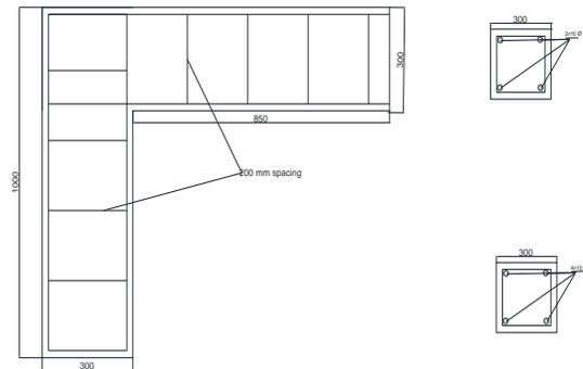
Fig. 3. L shape BC joint
