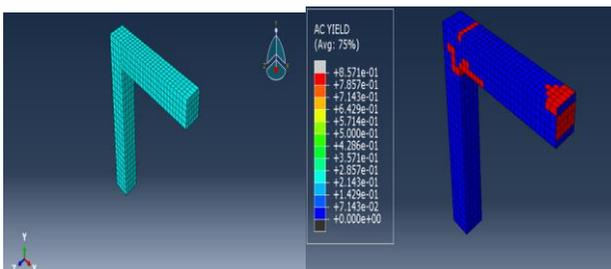
Fig. 7. Meshing and yielding of reinforcement and cracks in the model
