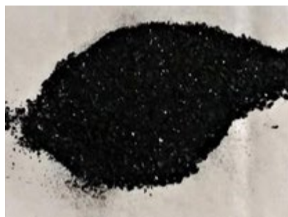
Fig. 4. Fe 2 O 3 nanoparticles after annealing
