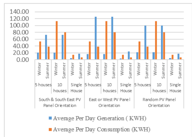
Fig. 5. Weekly average summer and winter energy Generation (kWh) and Consumption (kWh) for 5 Houses, 10 Houses and single House Community from the PV systems installed on various orientations
