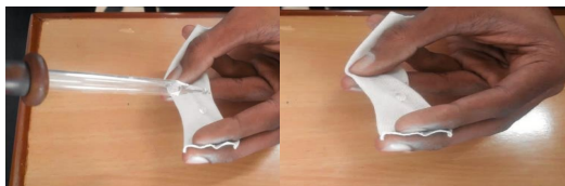
Fig. 4. Water observation trail (untreated fabric)
