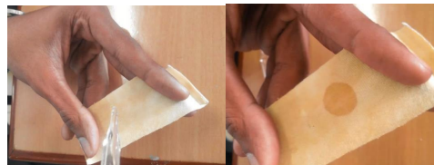
Fig. 5. Water observation trail (treated fabric)
