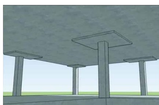
Fig. 2. Slab with drop
