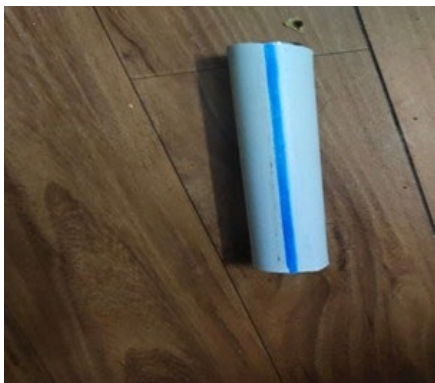
Fig. 2. PVC pipe used as roller
