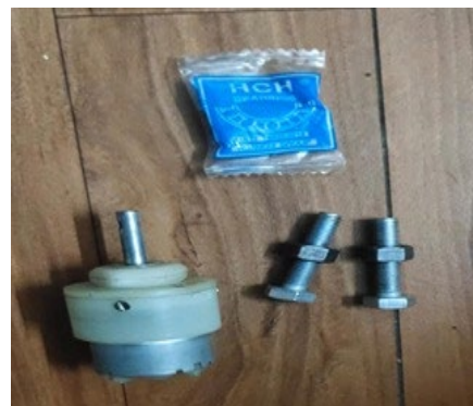
Fig. 1. 12V Stepper gear motor and nut and bolt
