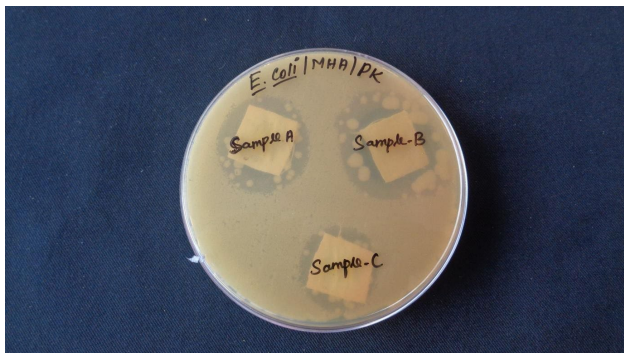
Fig. 6. Anti-Microbial activity – Concentration of 30 (gpl) Sample A, 40 (gpl) sample B, 50(gpl) sample C
