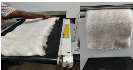
Fig. 5. Formation of nonwoven panel
