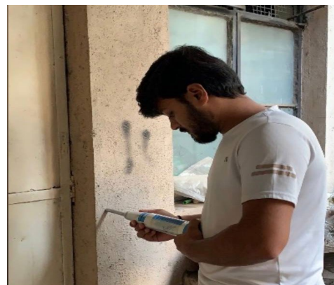
Fig. 6. Working of rebound hammer
