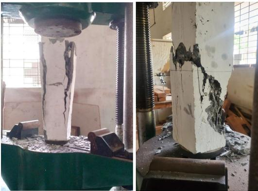
Fig. 9. Cracking pattern for retrofitting and conventional
