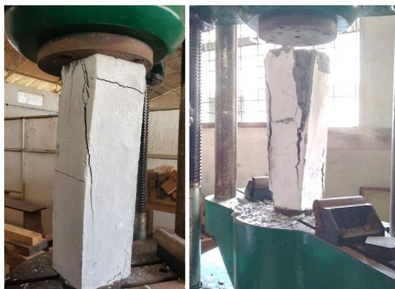
Fig. 5. Ultimate load of retrofitting
