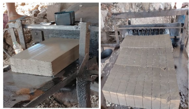
Fig. 2. Molding of brick
