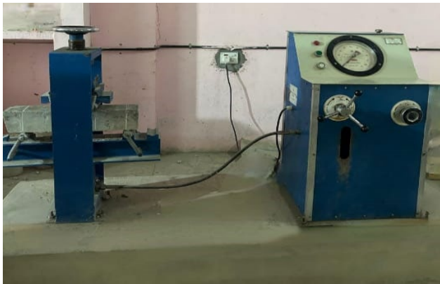
Fig. 3. Flexural strength test apparatus with specimen
