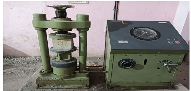
Fig. 1. Compressive strength test apparatus with specimen
