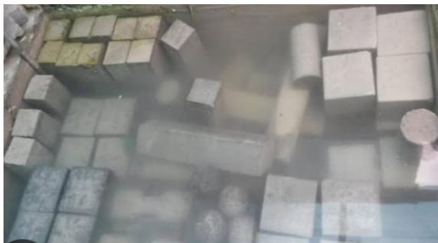
Fig. 4. Curing tank with specimen
