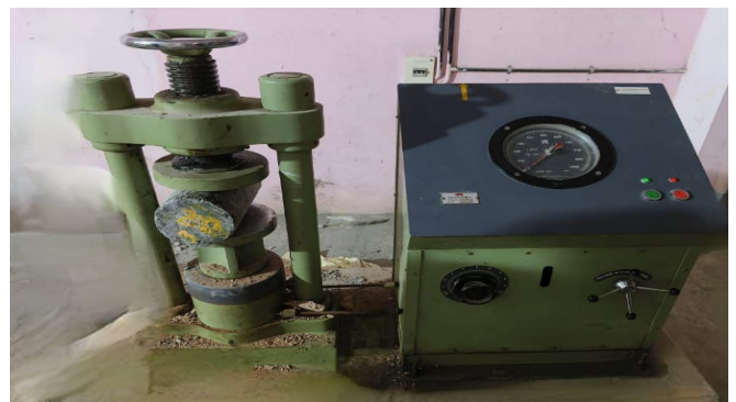
Fig. 2. Split tensile strength test apparatus with specimen
