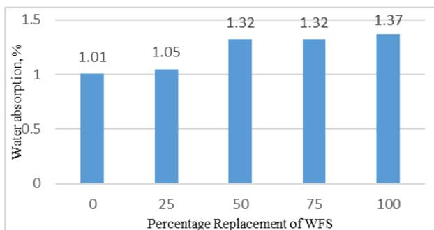
Fig. 8. Graph of 28days water absorption of cube
