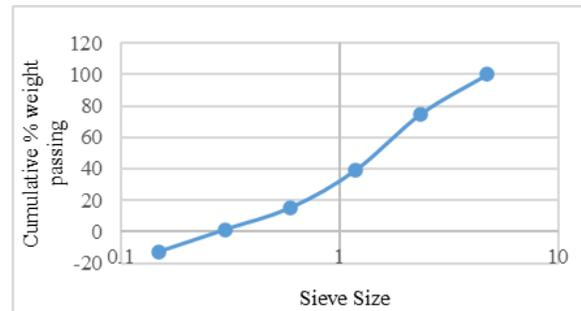
Fig. 3. Particle size distribution of M Sand
