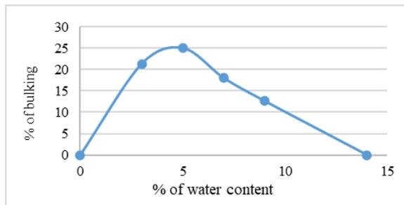
Fig. 1. Bulking of M Sand
