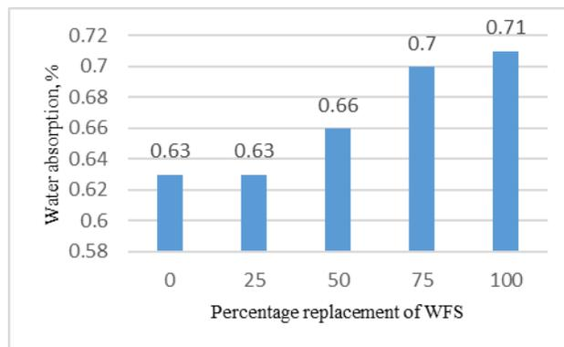
Fig. 10. 28days water absorption of beam
