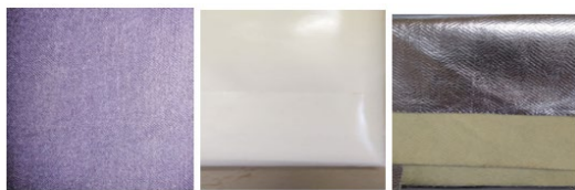
Outer layer as Nomex fabric Moisture barrier As PTFE coated Glass fiber fabric Thermal liner as Aluminized Kevlar fabric
