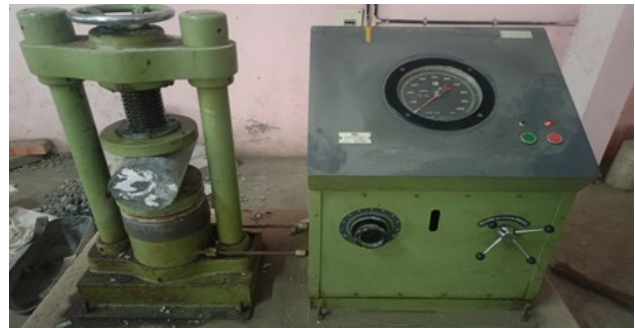
Fig. 9. Split tensile strength testing apparatus
