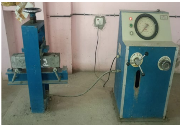
Fig. 7. Flexural strength testing apparatus
