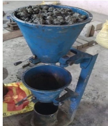
Fig. 4. Compaction factor test
