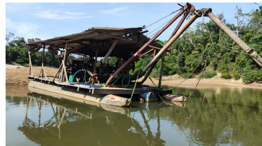
Fig. 1. Sand dredging process in the Jamari Valley, RO Source: Authors, 2025
