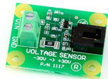
Fig. 3. Commercial voltage-sensor module (a current-sensor module follows the same principle)
