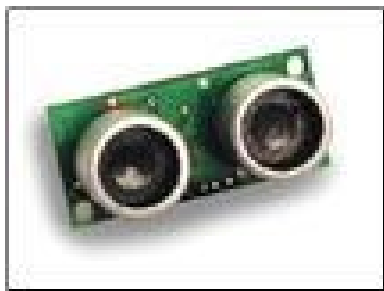
Fig. 6. Ultrasonic sensor module used for oil-level sensing
