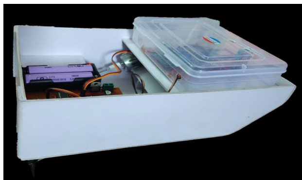
Fig. 6. Assembled RC boat prototype with sensing and navigation electronics
