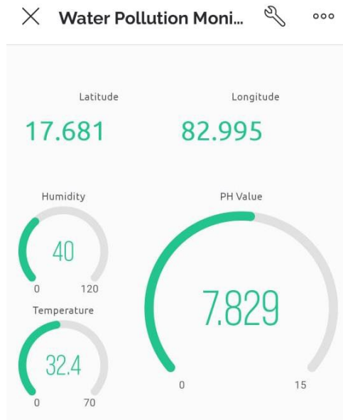
Fig. 7. Blynk application dashboard showing live GPS, humidity, temperature and pH readings
