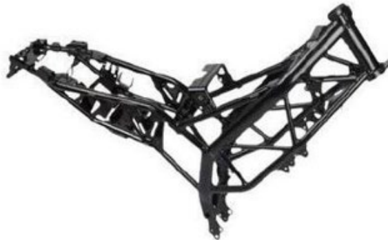
Fig. 3. Double cradle (twin-down-tube) chassis (e.g. Ather 450X, Royal Enfield Continental GT650)
