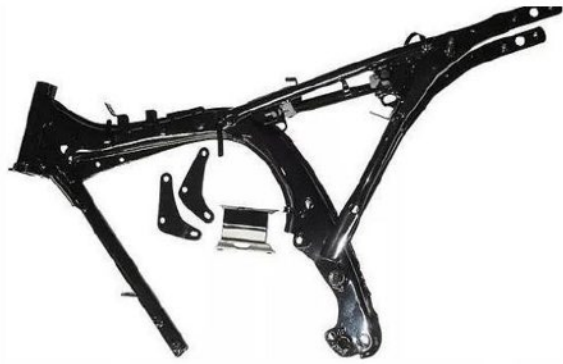
Fig. 2. Single cradle (single down-tube) chassis (e.g. Honda CG125, TVS Victor)
