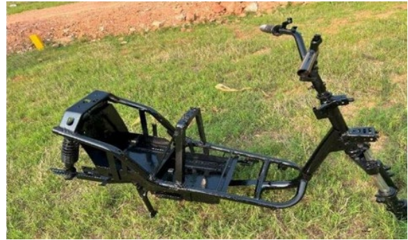
Fig. 5. Fabricated double-cradle chassis of the prototype two-wheeler EV
