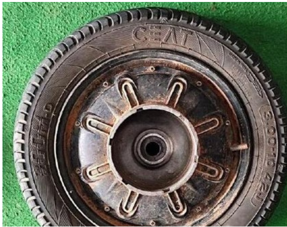
Fig. 12. Rear wheel and hub assembly of the fabricated prototype
