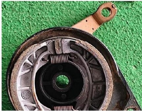
Fig. 13. Rear drum-brake assembly used on the prototype
