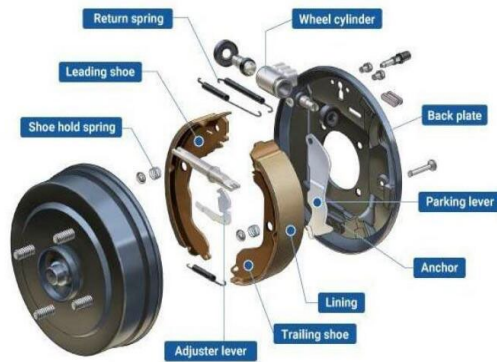
Fig. 9. Exploded view of a drum-brake assembly: drum, shoes, springs, backplate and wheel cylinder
