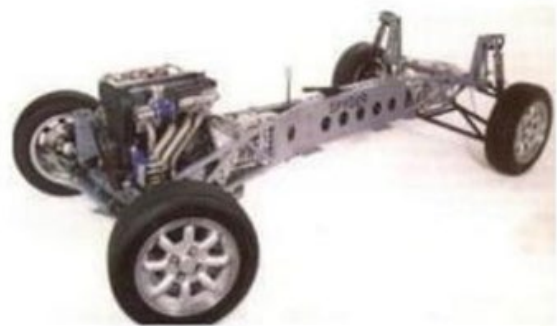
Fig. 1. Backbone chassis - A single spine running along the centreline (e.g. Honda CD100)
