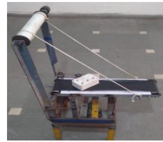
Fig. 7. Four axis conveyer belt
