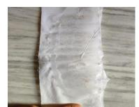
Fig. 5. Epoxy resin sample by padding method of bleached fabric
