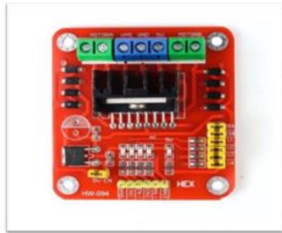
Fig. 5. L298N dual H Bridge Module
