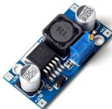
Fig. 7. XL6009 Step up boost converter
