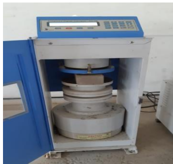
Fig. 6. Compression test on foundry sand brick
