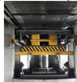
Fig. 3. Casting raw materials into bricks
