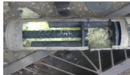
Fig. 1. Standard assembly of muffler
